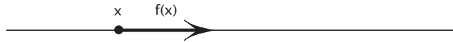
Figure 3.1: Interpreting the ODE \dot{x} = f(x) as a vector field on the line.
